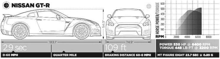
PRICE: \$90,950 DRIVELINE: Front engine/3.8L/530-hp/448-lb-ft twin-turbo V-6/7T-cl A/AWD SUSPENSION, F;R: Control arms, coil springs, adj shocks, anti-roll bar; multilink, coil springs, adj shocks, anti-roll bar BRAKE DISCS/CLPRS, F;R 15.4-in vented, drilled disc; 15.0-in vented, drilled disc; ABS CURB WEIGHT (DIST F/R) 3894 lb (55/45%) TIRES, F;R 255/40ZRF20 97Y; 285/35ZRF20 100Y Dunlop SP Sport Maxx CT 600 DSST CTT
