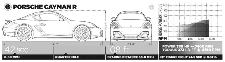
PRICE: \$78,150 DRIVELINE: Mid-engine/3.4L/330-hp/273-lb-ft flat-6/7t-cl.A/RWD SUSPENSION, F;R: Struts, coil springs, anti-roll bar; struts, coil springs, anti-roll bar BRAKE DISCS/CLPRS, F;R 12.5-in vented, drilled disc/6-piston; 11.8-in vented, drilled disc/4-piston, ABS CURB WEIGHT (DIST F/R) 3083 lb (45/55%) TIRES, F;R 235/35ZR19; 265/35ZR19 Bridgestone Potenza RE050A
