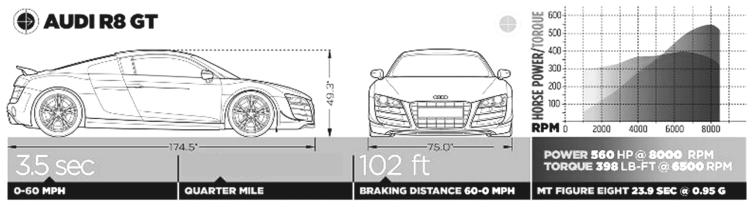
PRICE: \$200,100 DRIVELINE: Mid-engine/5.2L/560-hp/398-lb-ft V-10/6A-cl M/AWD SUSPENSION, F;R: Control arms, coil springs, adj shocks, anti-roll bar; control arms, coil springs, anti-roll bar BRAKE DISCS/CLPRS, F:R 15.0-in vented, drilled carbon-ceramic disc/6-piston; 14.0-in vented, drilled carbon-ceramic disc/4-piston, ABS CURB WEIGHT (DIST F/R) 3484 lb (43/57%) TIRES, F;R 235/35ZR19 91Y; 305/30ZR19 102Y Pirelli PZero Corsa
