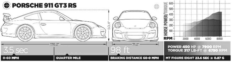
PRICE: \$149,820 DRIVELINE: Rear engine/3.8L/450-hp/317-lb-ft flat-6/6M/RWD SUSPENSION, F;R: Control arms, coil springs, adj shocks, adj anti-roll bar; multilink, coil springs, adj shocks, adj anti-roll bar BRAKE DISCS/CLPRS, F;R 15.0-in vented, drilled carbon-ceramic disc/6-piston; 13.8-in vented, drilled carbon-ceramic disc/4-piston, ABS CURB WEIGHT (DIST F/R) 3157 lb (39/61%) TIRES, F;R 245/35ZR19 89Y; 325/30ZR19 101Y Michelin Pilot Sport Cup
