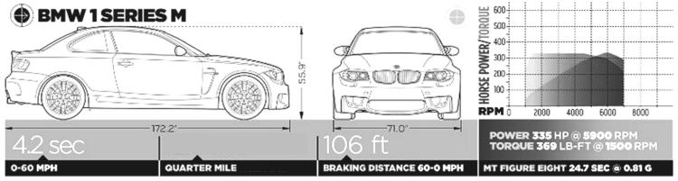
PRICE: \$50,460 DRIVELINE: Front engine/3.0L/335-hp/332-lb-ft\* twin-turbo I-6/6M/RWD SUSPENSION, F;R: Struts, coil springs, anti-roll bar; multlink, coil spring, anti-roll bar BRAKE DISCS/CLPRS, F;R 14.2-in vented, drilled disc/1-piston; 13.8-in vented, drilled disc/1-piston, ABS CURB WEIGHT (DIST F/R) 3402 lb (51/49%) TIRES, F;R 245/35ZR19 93Y; 265/35ZR19 98Y Michelin Pilot Sport PS2 \*(369-lb-ft w/overboost)
