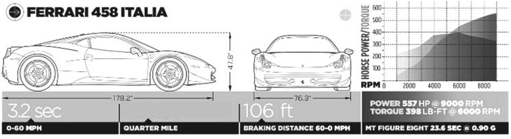
PRICE: \$287,654 DRIVELINE: Mid-engine/4.5L/557-hp/398-lb-ft V-8/7T-cl A/RWD SUSPENSION, F;R: Control arms, coil springs, adj shocks, anti-roll bar; multilink, coil springs, adj shocks, anti-roll bar BRAKE DISCS/CLPRS, F;R 15.7-in vented, drilled carbon-ceramic disc/6-piston; 14.2-in vented, drilled carbon-ceramic disc/4-piston, ABS CURB WEIGHT (DIST F/R) 3440 lb (43/57%) TIRES, F;R 235/35ZR20 92Y; 295/35ZR20 101Y Michelin Pilot Super Sport K1
