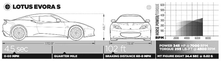
PRICE: \$90,110 DRIVELINE: Mid-engine/3.5L/345-hp/295-lb-ft supercharged V-6/6M/RWD SUSPENSION, F;R: Control arms, coil springs, anti-roll bar; control arms, coil springs, anti-roll bar BRAKE DISCS/CLPRS, F:R 13.8-in vented, drilled disc/4-piston; 13.1-in vented, drilled disc/4-piston, ABS CURB WEIGHT (DIST F/R) 3171 lb (39/61%) TIRES, F;R 235/35ZR19 91Y; 275/30ZR20 97Y Pirelli PZero Corsa
