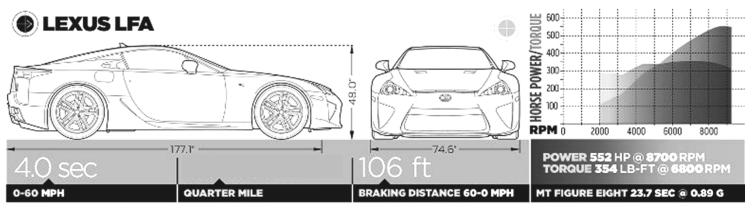
PRICE: \$381,100 DRIVELINE: Front engine/4.8L/552-hp/354-lb-ft V-10/6A-cl M/RWD SUSPENSION, F;R: Control arms, coil springs, anti-roll bar; multilink, coil springs, anti-roll bar BRAKE DISCS/CLPRS, F;R 15.4-in vented, drilled carbon-ceramic disc/6-piston; 14.2-in vented, drilled carbon-ceramic disc/4-piston, ABS CURB WEIGHT (DIST F/R) 3559 lb (50/50%) TIRES, F;R 265/35ZR20 95Y; 305/30ZR20 99Y Bridgestone Potenza S001
