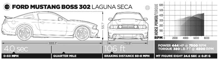
PRICE: \$48,100 DRIVELINE: Front engine/5.0L/444-hp/380-lb-ft V-8/6M/RWD SUSPENSION, F;R: Struts, coil springs, adj shocks, anti-roll bar; live axle, coil springs, adj shocks, anti-roll bar BRAKE DISCS/CLPRS, F:R 14.0-in vented disc/4-piston; 11.8-in vented disc/1-piston, ABS CURB WEIGHT (DIST F/R) 3640 lb (55/45%) TIRES, F;R 255/40ZR19; 285/35ZR19 Pirelli PZero Corsa
