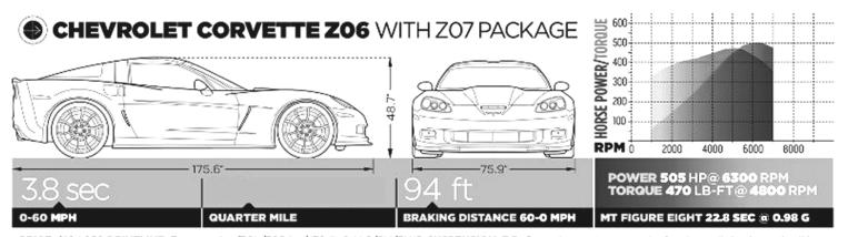
PRICE: \$104,650 DRIVELINE: Front engine/7.0L/505-hp/470-lb-ft V-8/6M/RWD SUSPENSION, F;R: Control arms, transverse leaf spring, adj shocks, anti-roll bar; control arms, transverse leaf spring, adj shocks, anti-roll bar BRAKE DISCS/CLPRS, F:R 15.5-in vented, drilled carbon-ceramic disc/6-piston; 15.0-in vented, drilled carbon-ceramic disc/4-piston, ABS CURB WEIGHT (DIST F/R) 3320 lb (49/51%) TIRES, F;R 285/30ZR19 87Y; 335/35ZR20 94Y Michelin Pilot Sport Cup ZP
