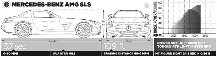
PRICE: \$205,200 DRIVELINE: Front engine/6.2L/563-hp/479-lb-ft V-8/7T-cl A/RWD SUSPENSION, F;R: Control arms, coil springs, anti-roll bar; control arms, coil springs, anti-roll bar BRAKE DISCS/CLPRS, F;R 15.4-in vented, slotted, drilled disc/6-piston; 14.2-in vented, slotted, drilled disc/4-piston, ABS CURB WEIGHT (DIST F/R) 3795 lb (46/54%) TIRES, F;R 265/35ZR19 98Y; 295/30ZR20 101Y Continental ContiSportContact 5P
